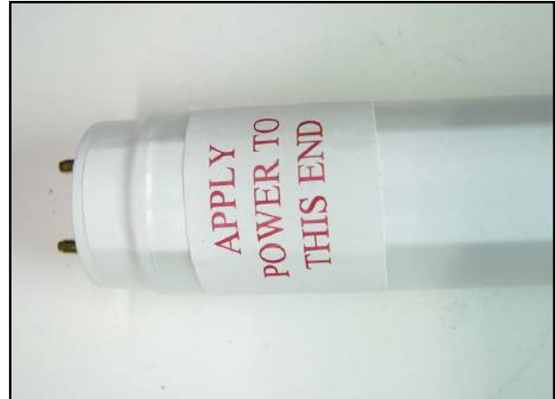
Figure 3 – Ballast bypass LED tubes must be installed so that they receive 120v AC on the labeled end.
