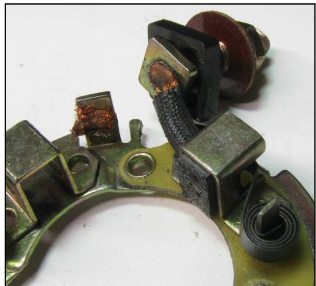
Figure 1 – Notice the arcing marks on the face of this worn out positive brush.
