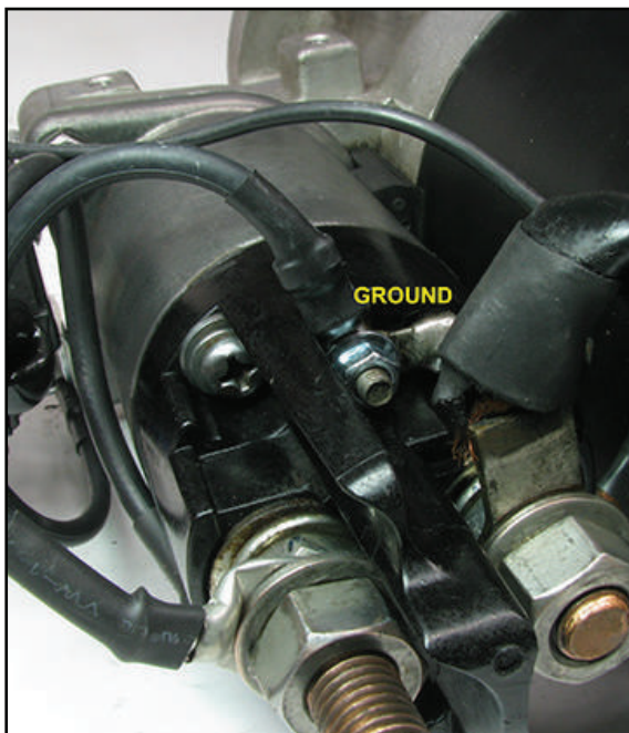
Figure 6 – Smart IMS ground wire connected to the solenoids ground.
