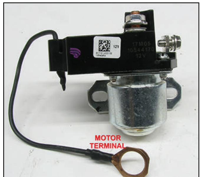
Figure 4 – Smart IMS with motor terminal connection.
