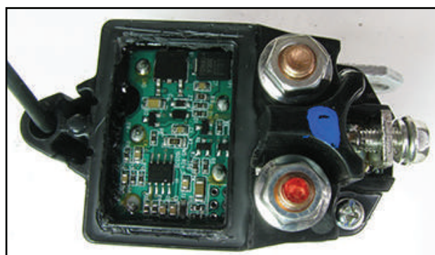
Figure 7 – View of the Smart IMS circuit board that has complete control of the switch.
