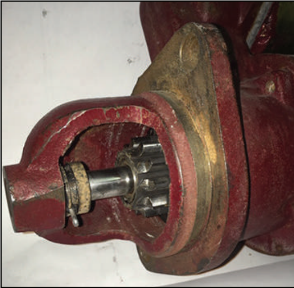
Figure 7 – The unknown Chinese starter with damaged drive
