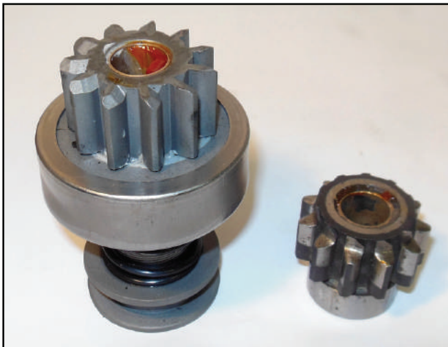
Figure 8 – The rebuilt drive by The Drive Doctor
