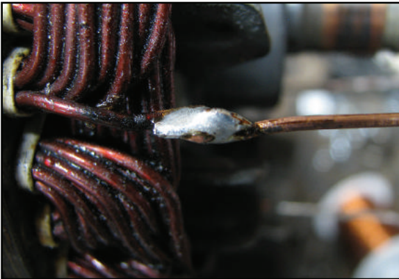
Figure 6 – The application of solder completes the repair.
