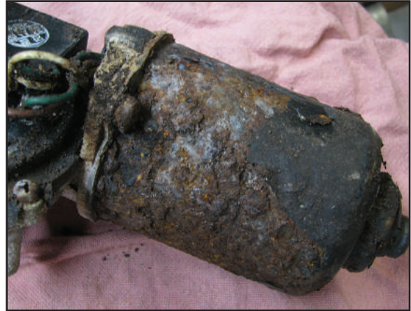
Figure 1 – This wiper motor mounts under the cowling on a Santa Fe, where it is exposed to moisture every time it rains.
