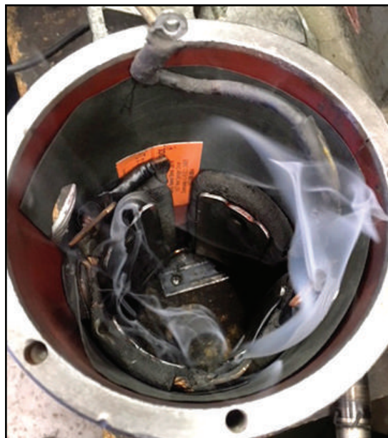
Figure 3 – Developed smoke under Hi-Voltage testing.
