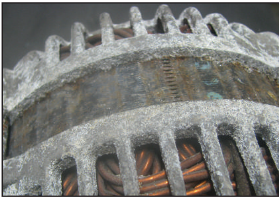
Figure 3 – This alternator has been exposed to moisture laden air and is covered with hydrated aluminum oxide.
