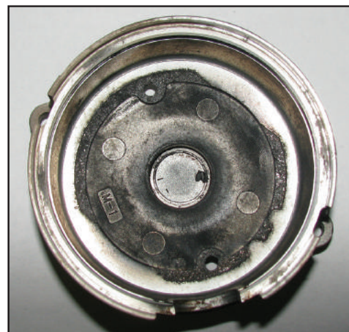
Figure 6 – This is the Duramax starter's aluminum CE housing with a matching ring of missing material.
