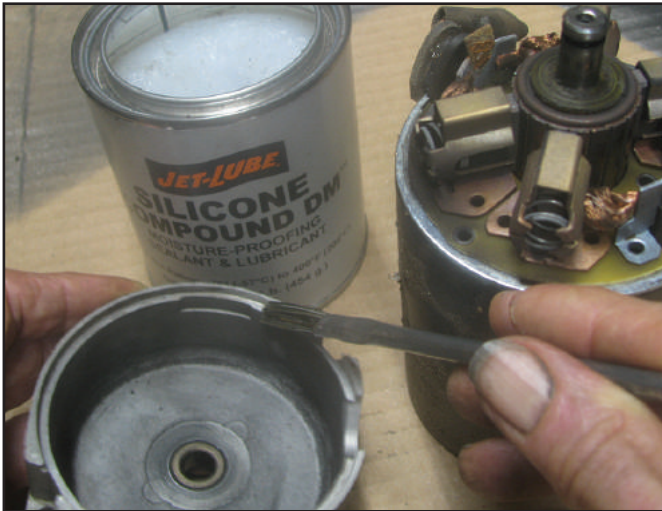
Figure 7 – The application of dielectric grease to the contact surface on this Bosch CE will fill any air gaps that might accumulate moisture.
