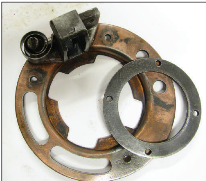
Figure 10 – The steel ring with four threaded holes effectively clamps the adjustable brush holder assembly to the end frame.
