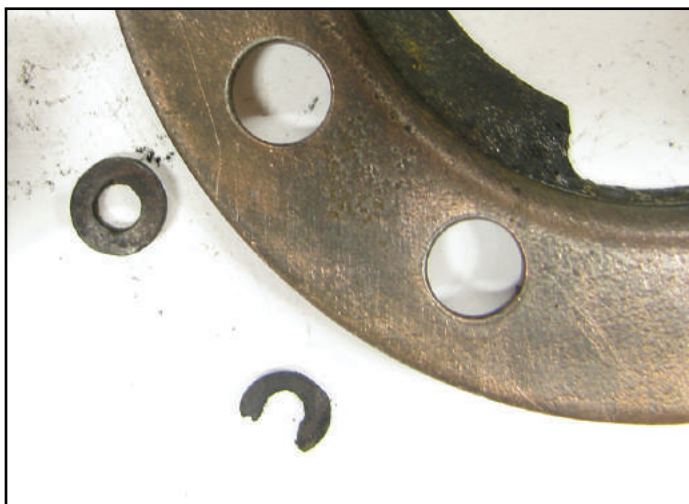
Figure 6 – That is not a C-clip on the lower right. It is what was left of the round rivet insulator.
