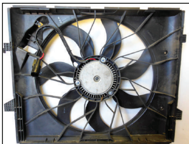
Figure 4 – A Chrysler Radiator Cooling Fan with Brushless DC Motor
