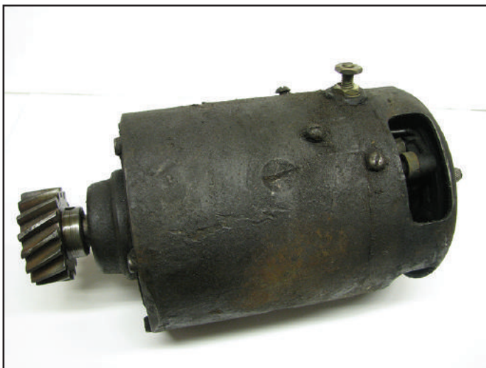
Figure 1 – Gear-driven Model T Ford generator – 6 volt, negative ground.
