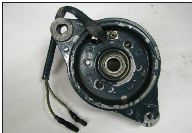
Figure 11 – The rear bearing must be knocked out of the back side of the stator frame.
