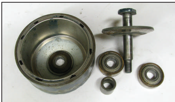
Figure 10 – One bolt holds all of these rotor pieces together and attached to the stator frame.
