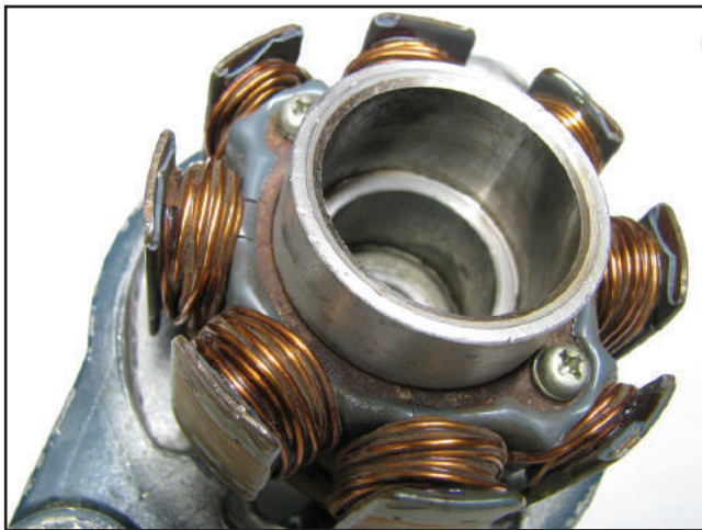
Figure 5 – The eight coils are wound in series from one continuous piece of wire, resulting in two leads.
