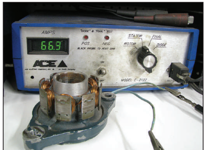
Figure 7 – A stator tester verified continuity under load and allowed a short to ground test by moving one lead to a steel surface.
