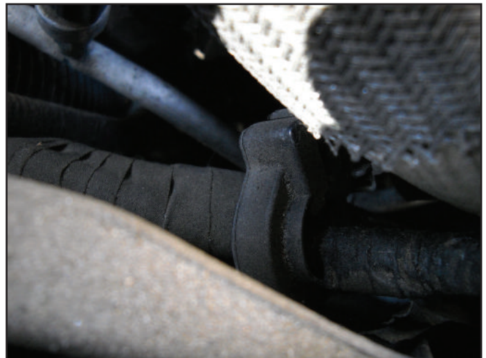
Figure 2 – Ford's alternator current sensor in the F150 is located out view, under the upper radiator hose.
