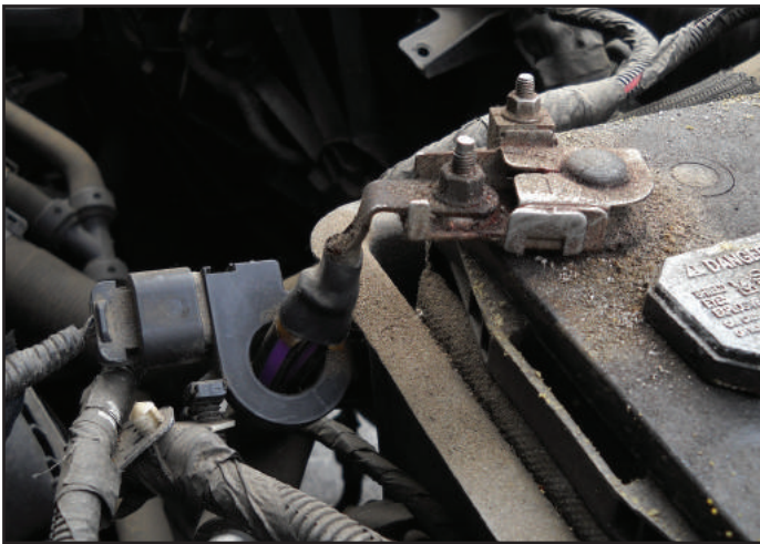
Figure 1 – This current sensor on the negative battery cable is a key part of Ford's Battery Monitoring System.
