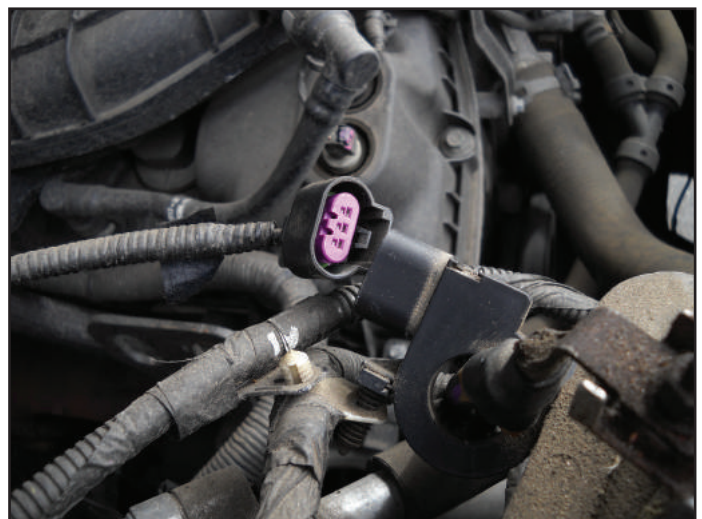
Figure 3 – Ford's current sensors utilize three wires as you can see in this familiar looking Ford plug connection.
