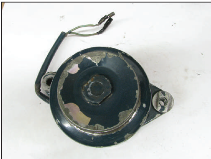
Figure 1 – The most common Denki alternators look like this one.
