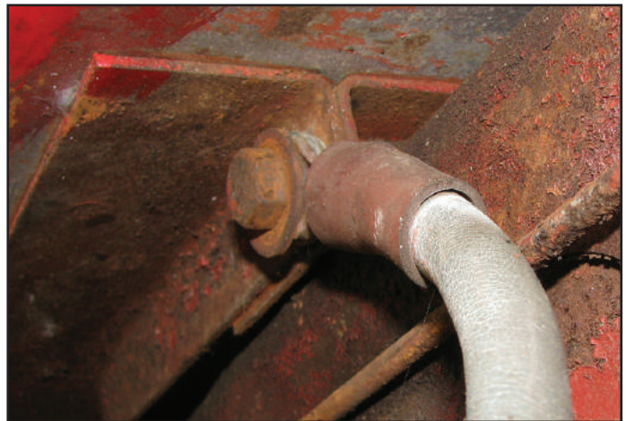
Figure 3 – The negative battery cable was bolted to a bracket under the fuel tank, above and behind the battery.
