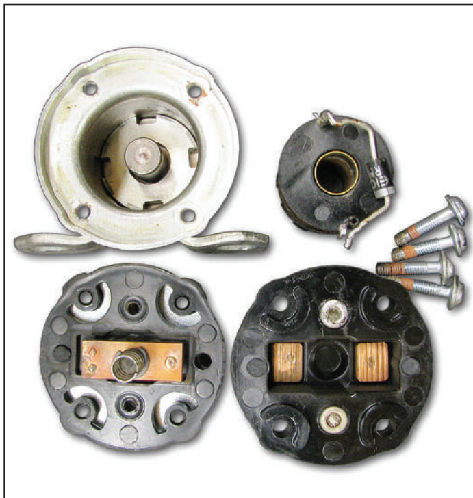
Figure 17 – This is a disassembled Delco-Remy IMS (Integrated Magnetic Switch).
