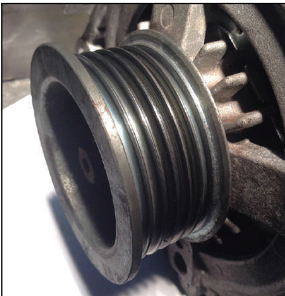
Figure 3 - A close inspection of the pulley reveals abnormal wear on the center surfaces.
