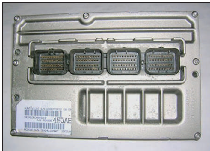
Figure 3 – Next Generation Controller (NGC). Note: Four 38-pin Connectors
