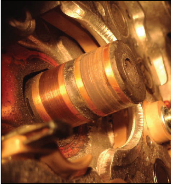
Figure 4 – Notice here that the outer slip ring shows signs of significant arcing.
