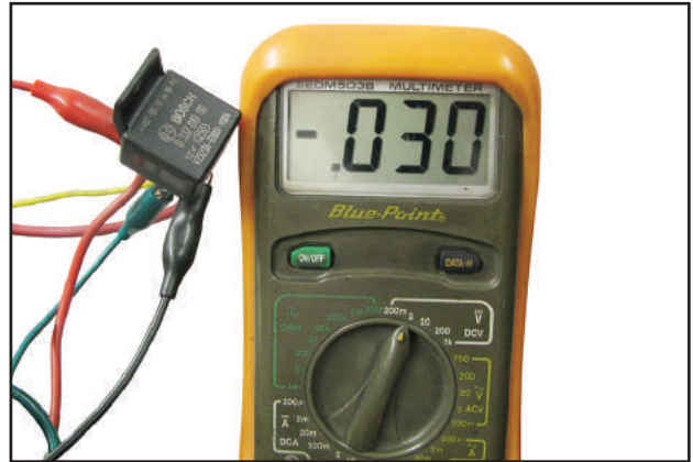
Figure 10 – The voltage drop shown here was taken with a 20-amp load on the relay.
