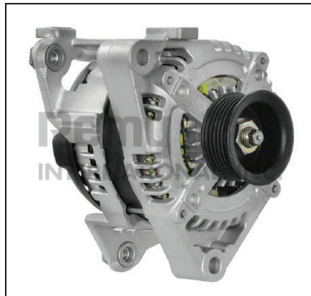
Figure 1 - Denso Alternator 104210-3280, used on 2000-03 Cadillac CTS vehicles with 3.2L engine.
