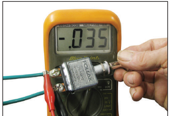
Figure 6 – The voltage drop here was made while momentarily overloading the switch by flowing 110 amps through it.
