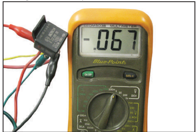
Figure 11 – The voltage drop here was taken with 40-amp load on the relay.
