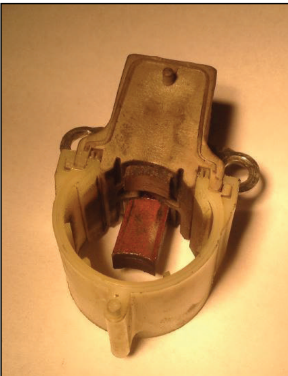
Figure 5 – Likewise, the outer brush was hot enough to melt the brush holder.
