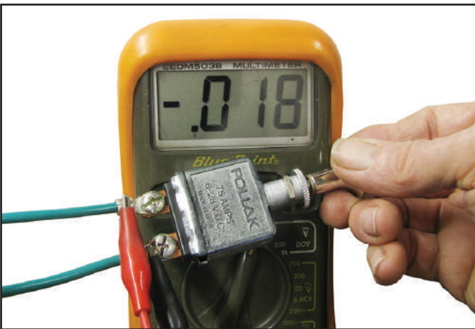
Figure 5 – The voltage drop shown here was made while passing 75 amps through the contacts.
