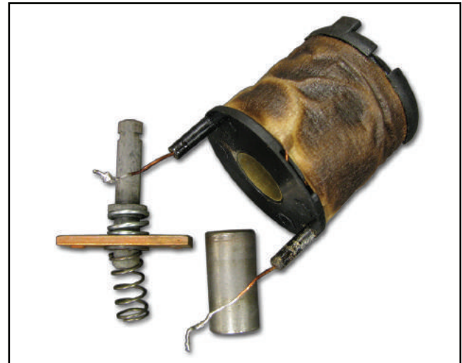
Figure 18 – This is a closer view of the coil, plunger and moving contact.
