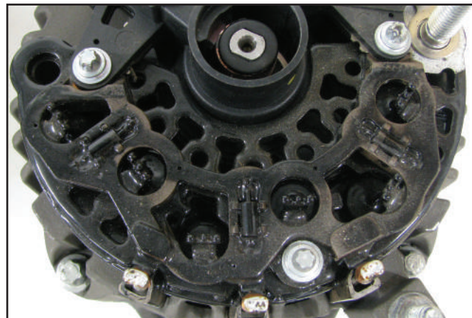
Figure 3 – The 11SI rectifier contains an integrated diode trio on the lead frame.
