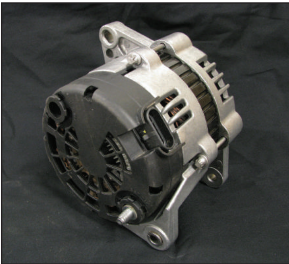
Figure 5 – The KD11's rear plastic cover has cosmetic differences from the 11SI but mounts identically.
