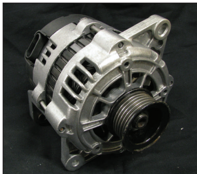
Figure 4 – Delco's KD11 alternator can be easily confused with an 11SI.
