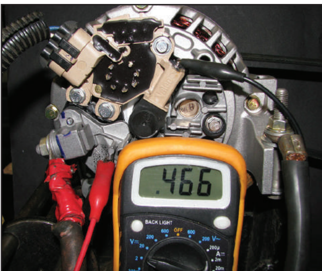
Figure 4 – The Vsat of this new GM/Valeo regulator is 0.46 volts, about what you would expect from a healthy regulator.
