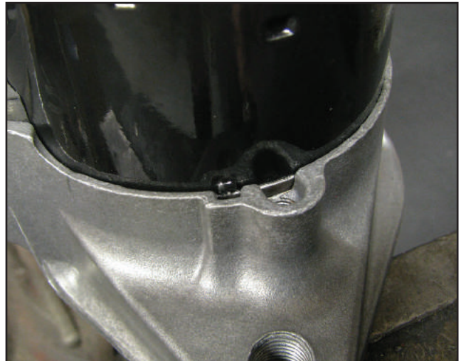
Figure 16 – Make sure that the locator bump on the field case is aligned and seated into the DE housing's indent.
