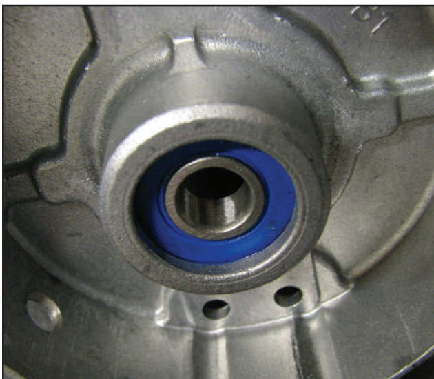
Figure 11 – The 608 ball bearing must be fully seated in the CE frame to insure proper armature positioning.
