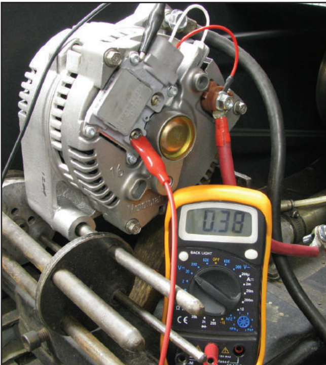
Figure 3 – The Vsat on this aftermarket 3G regulator is well within limits at 0.38 volts.
