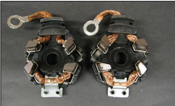
Figure 5 – The brushes are trapezoid-shaped and slanted to match the spiral commutator bars.
