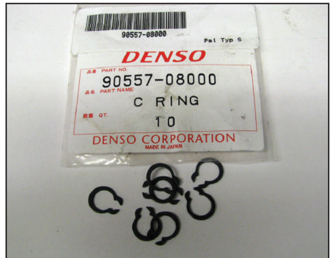
Figure 8 – Denso offers the snap ring as a service part. I highly recommend that you keep them on hand.
