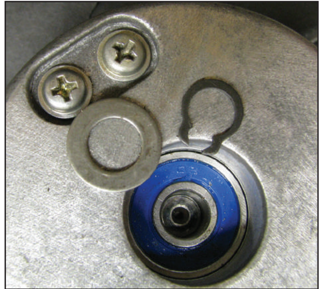
Figure 7 – This small snap ring and spacer washer are both tiny and important parts.
