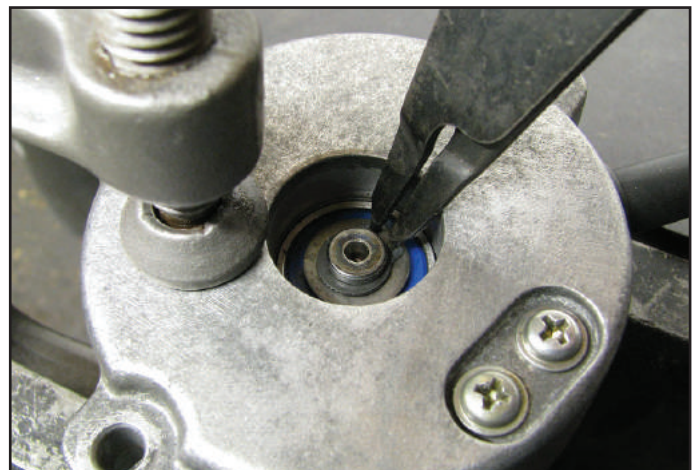
Figure 13 – The clamp allows two hands free to install the washer and snap ring.
