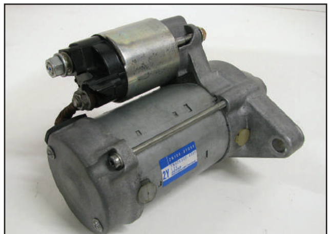
Figure 18 – Denso replaced the flat commutator starters with a newer version using a more conventional armature.
