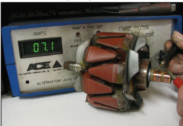
Figure 6 – Field draw on the low resistance (1.8 ohms) rotor is around 7 amps and goes with the 12-diode rectifier.
