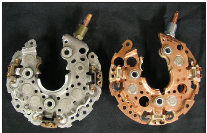
Figure 3 - The rectifier on the left, taken from 421000-0280, has 12 diodes. The seven diode rectifier is on the right.
