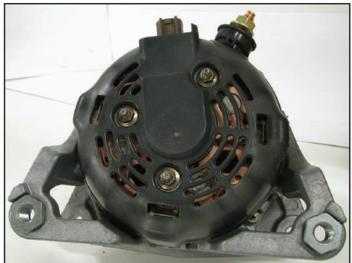
Figure 2 - From this view, you can identify it as 421000-0210 by its seven diode rectifier - if you look closely.
