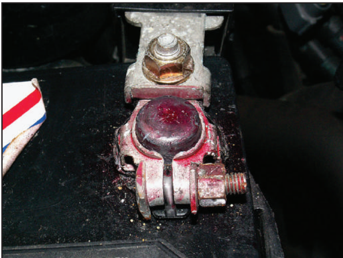
Figure 2 – This happens to be an OEM Nissan top-terminal setup. Once again, the terminal is fully seated on the battery post and a noticeable portion of the post sticks up above the terminal itself.
