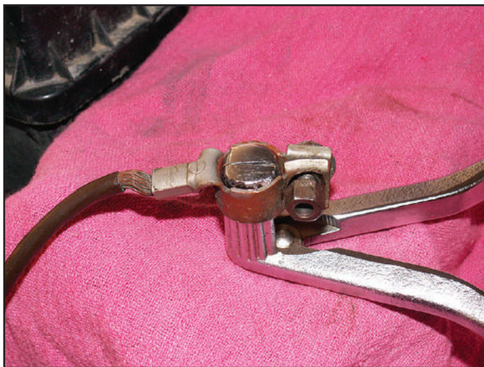
Figure 3 – Here, I am using the basic, pliers-shaped tool to carefully spread open a top-post battery terminal. No, this spreader tool isn't essential but I've found it to be inexpensive and efficient for the task.
