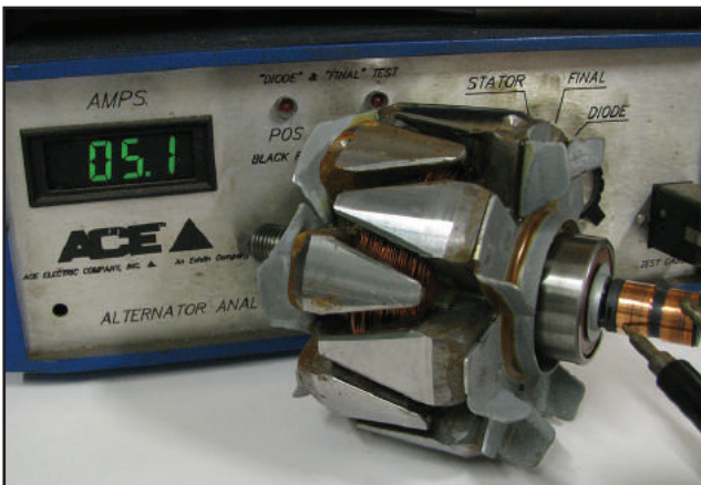
Figure 5 – Field draw on the higher resistance (2.5 ohms) rotor is around 5 amps and goes with the 7-diode rectifier.
