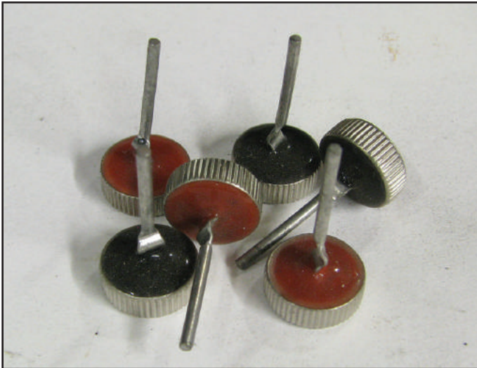
Figure 10 – The Denso press fit diodes have small stems which require good heat sinking technique when soldering them to the rectifier's lead frame.
