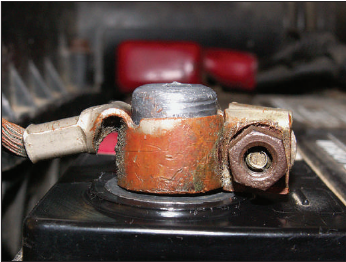
Figure 1 – This is a side view of a common Honda top-terminal battery terminal. I have loosened the nut, spread the terminal and then fully “seated” it on the post. Consequently, a noticeable portion of the post protrudes through the terminal.
