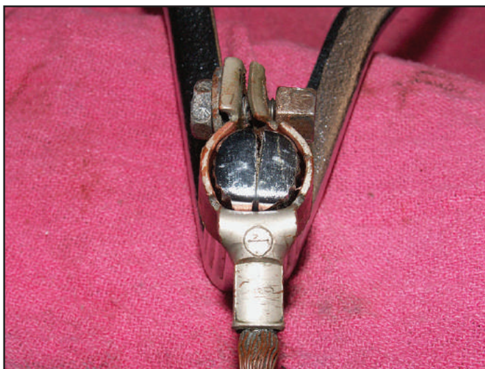
Figure 4 – This is just a closer view of the simple spreader tool at work. Naturally, it's preferable to spread a terminal just enough to fit fully onto the battery post – without distorting or damaging that terminal.
