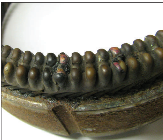
Figure 15 – The pattern suggests that one or two coils were heated to greatly higher temperatures.
