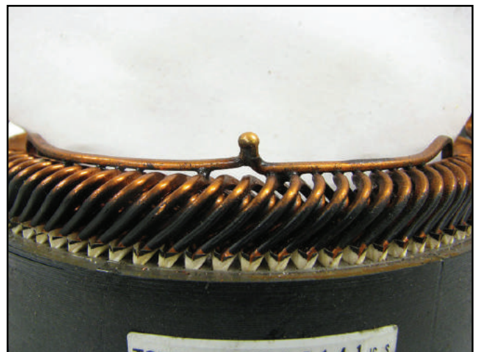
Figure 8 – Here you can see that the delta stator's series connection between two coils.
