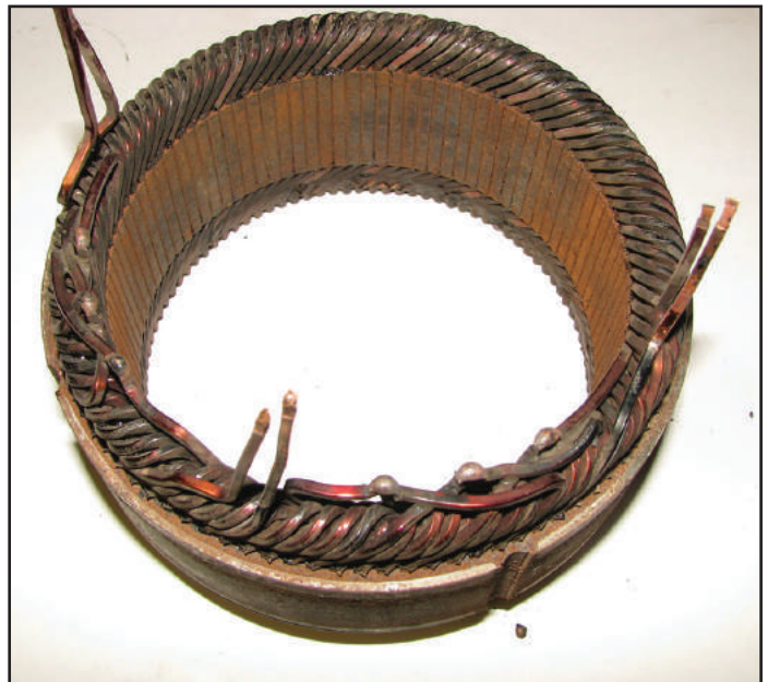
Figure 11 - This 138.5 mm 225 amp stator has obvious signs of overheating. Also notice that it has six spot welds with six lead wires.
