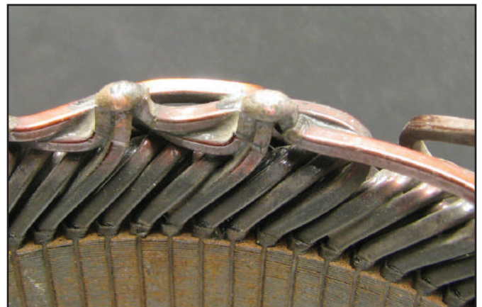
Figure 2 – The coils in a Denso SC stator can be spot welded into a variety of configurations – some unique and never used before.
