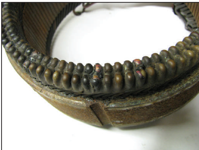
Figure 14 – A hot spot pattern is clearly visible in our burned stator sample.
