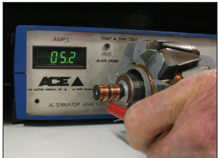
Figure 17 - Testing amperage draw here on the delta stator's rotor, we get a reading of 5.2 amps.
