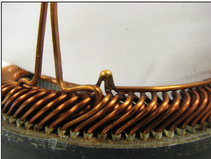
Figure 10 - Here you can see that the wye stator's connections join three coils, one for each phase.
