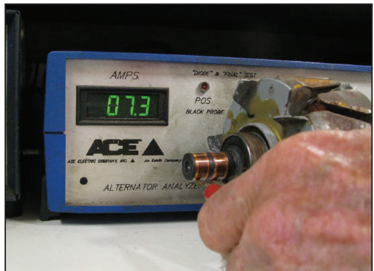
Figure 18 - Testing amperage draw on the wye stator's rotor, we get a reading of 7.3 amps which is significantly higher.
