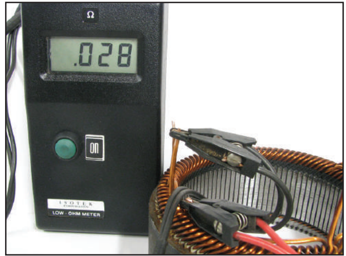
Figure 6 – Reading the resistance of one coil in the wye stator, between a lead and the wye spot weld, we get .028 ohm.
