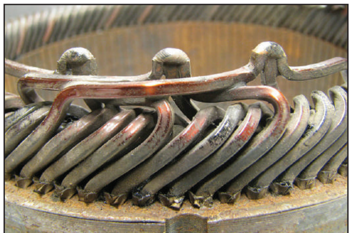
Figure 12 - Here you can see that each spot weld connects three coil ends.
