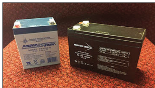
Figure 2 – These gel cell batteries were made for emergency backup service.
