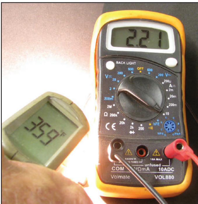
Figure 7 – Here you can see the current draw of the brake element of an 1157 bulb along with the its temperature after two minutes of “on” time, common in heavy traffic areas.
