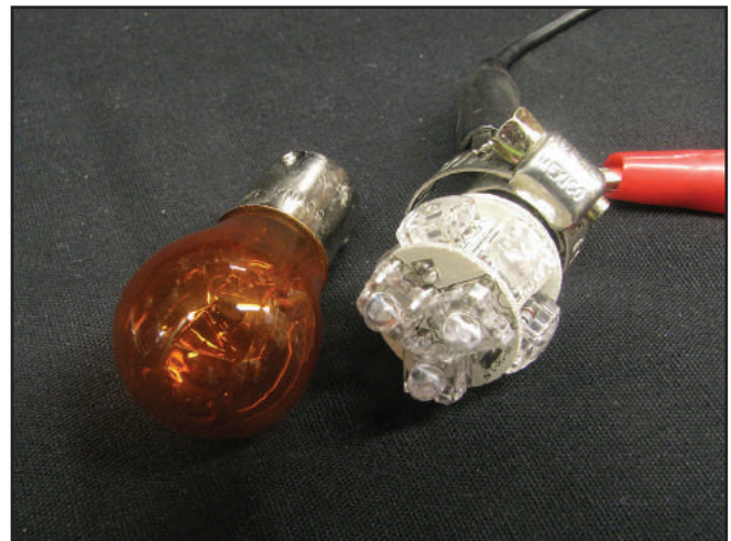
Figure 9 – This is an amber 1156 bulb next to a yellow LED lamp. Note that the LED lamp appears to be clear.
