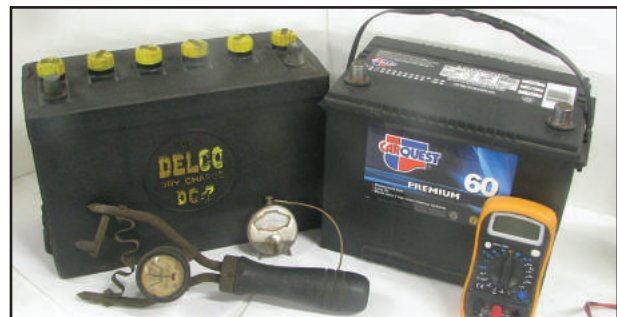
Figure 1 – This is a Delco cranking battery from the 1950's (left) compared to an East Penn made flooded wet cell cranking battery of today (right).
