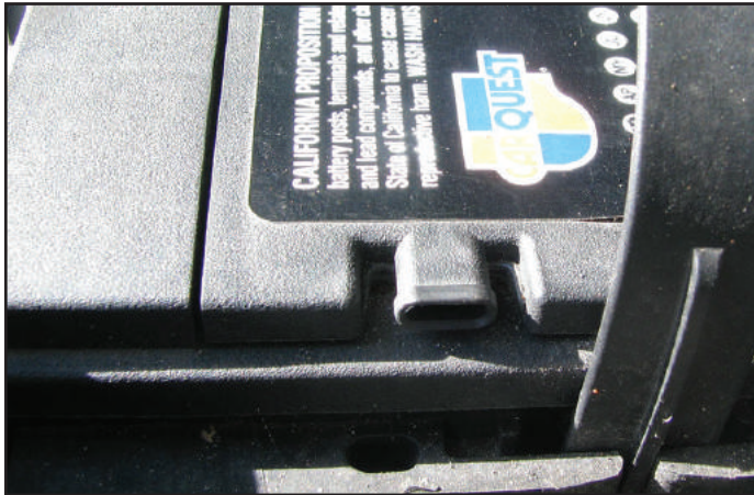
Figure 3 – Note that this flooded wet cell battery has the vent on the side of the cover.
