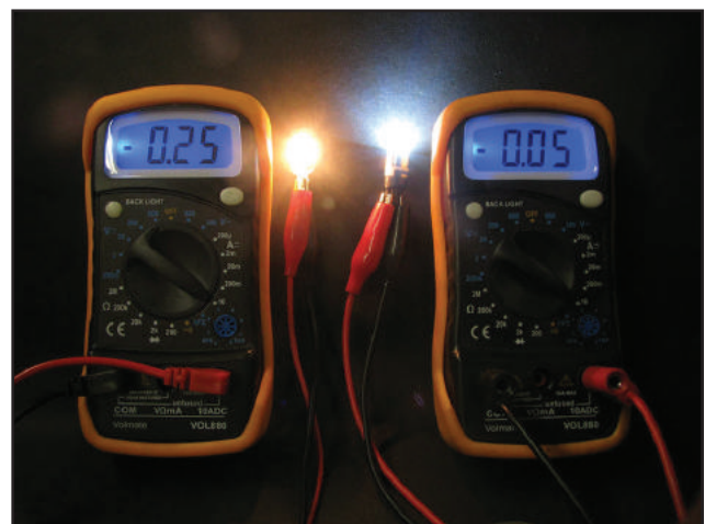
Figure 6 – Here you can see the brightness and the current draw between a standard 194 incandescent bulb (left) and its LED replacement (right) when powered with 14.5 volts. The LED is brighter on 80% less current.
