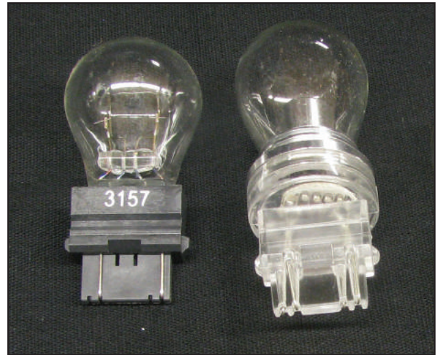
Figure 1 – Conventional tungsten 3157 tail/brake lamp (left) next to an 3157 LED replacement bulb (right).
