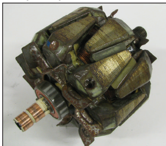
Figure 4 – This Valeo rotor has eight permanent magnets that are epoxied in four evenly spaced locations around the rotor.
