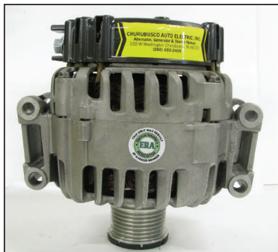
Figure 3 – This side view shows that the pad-mount bolt locations are not in a square pattern, making test bench mounting a challenge.
