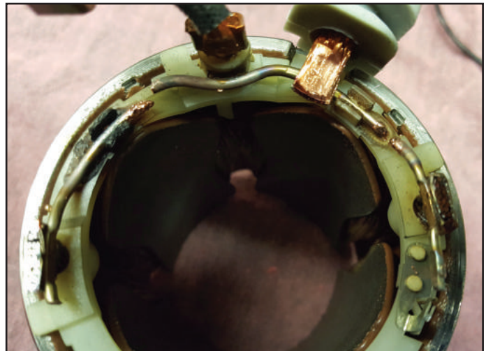
Figure 2 – Here you can see where they burned open on both sides of the field case lead.
