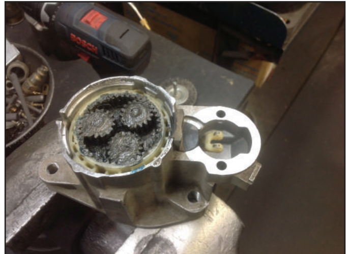
Figure 3 – Here you can see where the aluminum came from, taken from the drive end housing by galvanic corrosion.
