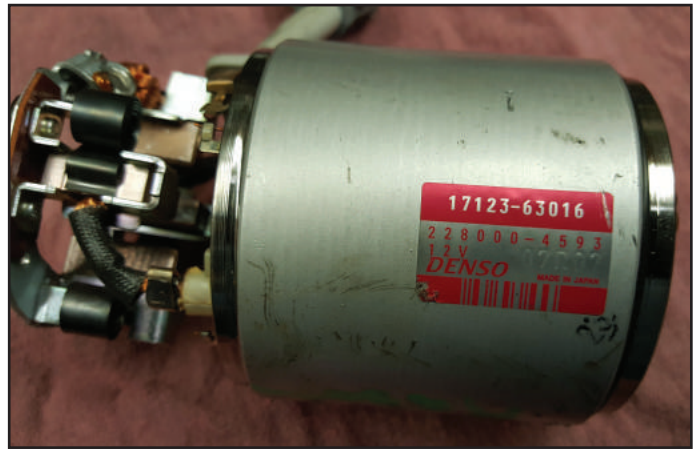
Figure 1 – This is the 2kW Denso field case with burned field coil lead wires.
