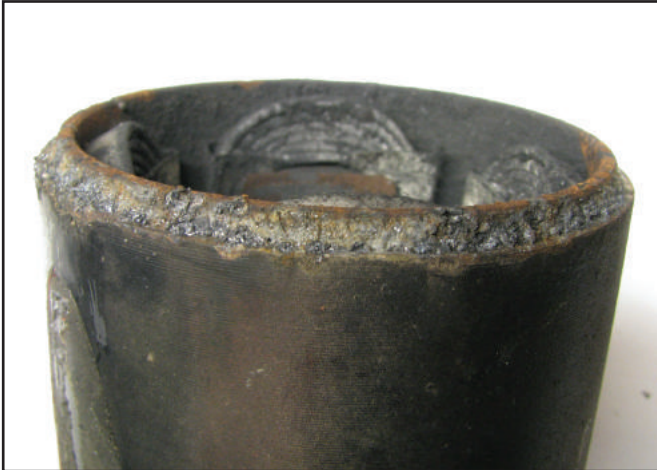
Figure 6 – Here you can see that the contact area on the steel field case is heavily coated with aluminum particles from the housing.
