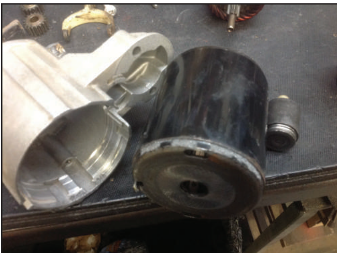
Figure 2– Note the aluminum that was deposited on the steel field case of this Mitsubishi Jeep starter.
