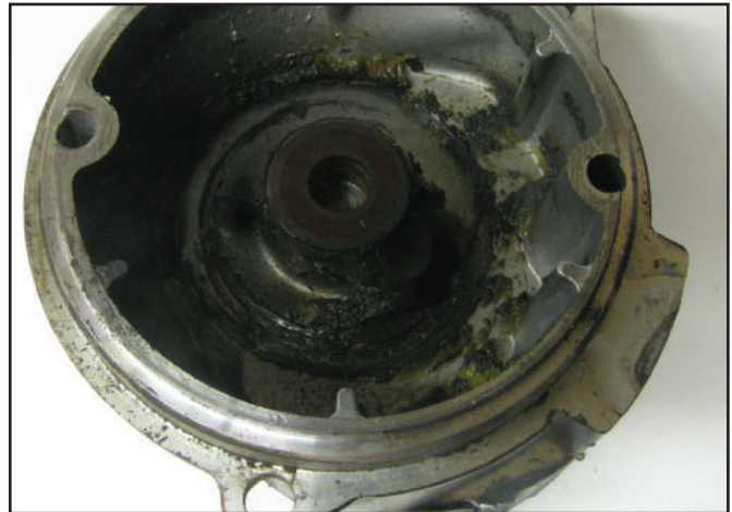
Figure 7 – The other side of the intermediate housing that was in contact with the aluminum drive end housing was in perfect condition.
