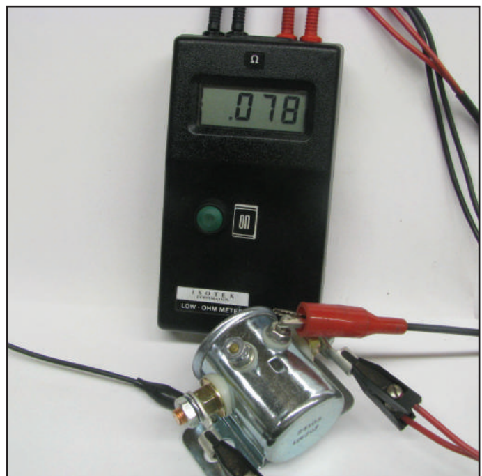
Figure 1 – Using a low ohm meter here, we are testing contact resistance of an external start relay.
