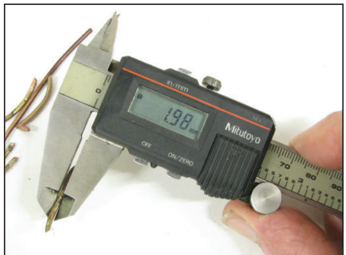
Figure 3 – Precise measurements are needed when replacing fuse wire.
