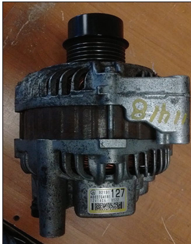
Figure 5 – Mitsubishi alternator used on the 2008 Pontiac G8 with RVC uses a clutch pulley.
