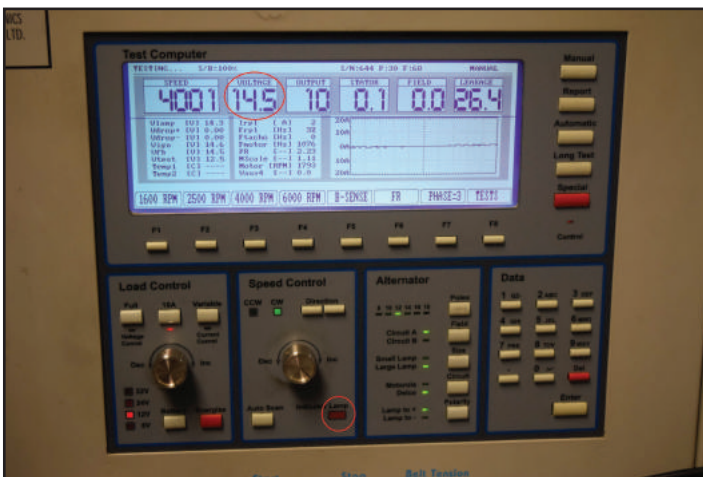
Figure 4 – This is the readout after excitation without any input to the C terminal. It is charging at the default rate of 14.5v.
