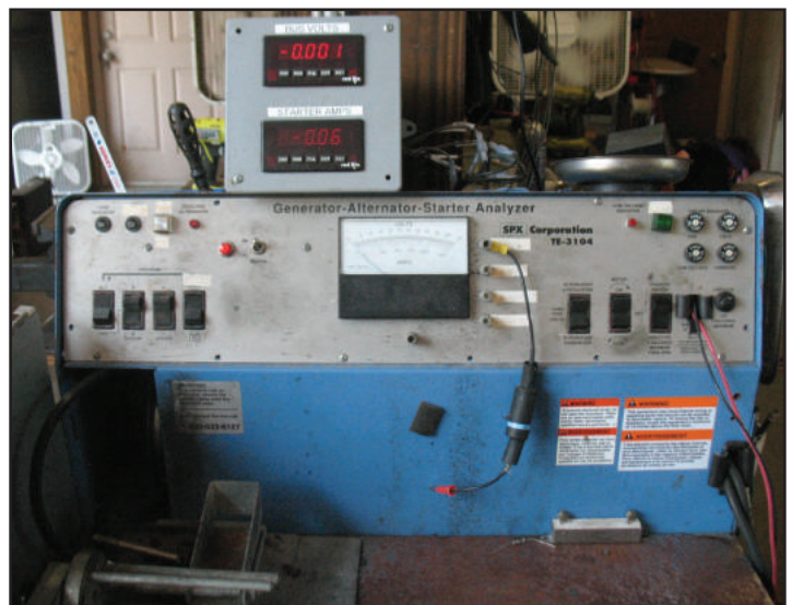
Figure 1 - This is a view of the Minitune bench after the upgrade. Notice the size of the display numerals on the digital panel compared to those on the original analog meter.
