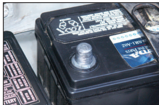
Figure 2 – This is common Honda battery terminal that I have cleaned and treated with a film of silicone paste. Years of experience has shown me that I remove the battery cables from this battery years from now, the battery post will still look just like this one.
