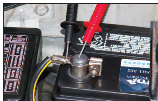
Figure 3 – Here, a helper cranks the engine while I hold one voltmeter lead on the battery post and the other lead on the battery terminal itself. Performing countless voltage drop tests just like this has shown me that the reading on a healthy connection is usually less than 0.10 volt. Beware, many battery connections that look good outside are actually corroded inside !
