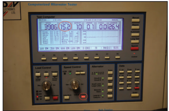
Figure 5 – This is the readout after B+ has been removed from the S terminal to test lamp operation. The regulator has entered secondary regulation because of the lack of sense voltage. Note that the indicator lamp has been turned on to indicate a problem.
